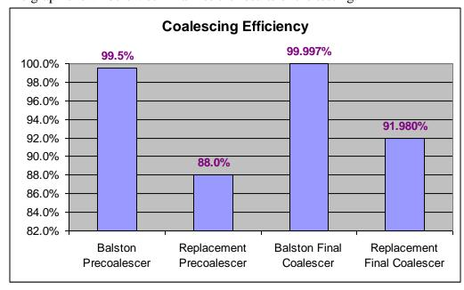
As you can see from the graph, the non-branded replacement filter elements did not meet or exceed the performance (or the specifications) of the Balston filter elements. In fact, the efficiency of the non-branded *final* coalescer was lower than the efficiency of the Balston *pre*coalescer!
